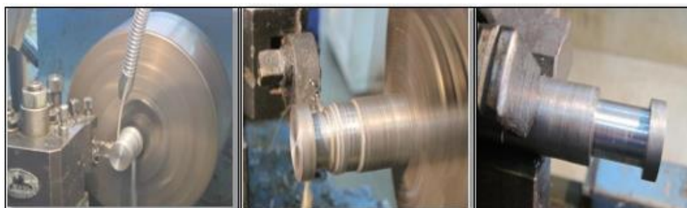
Figure 3.4: Facing Process on the Hand Crank Holder
