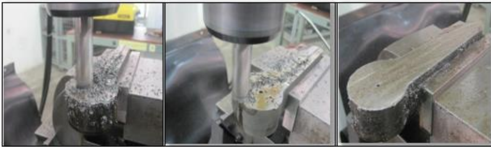
Figure 3.3: Material Surface Levelling Process
