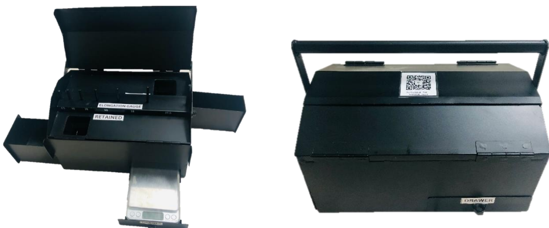
Figure 4: Elongation Test Kit 2.0 (ETK 2.0)
