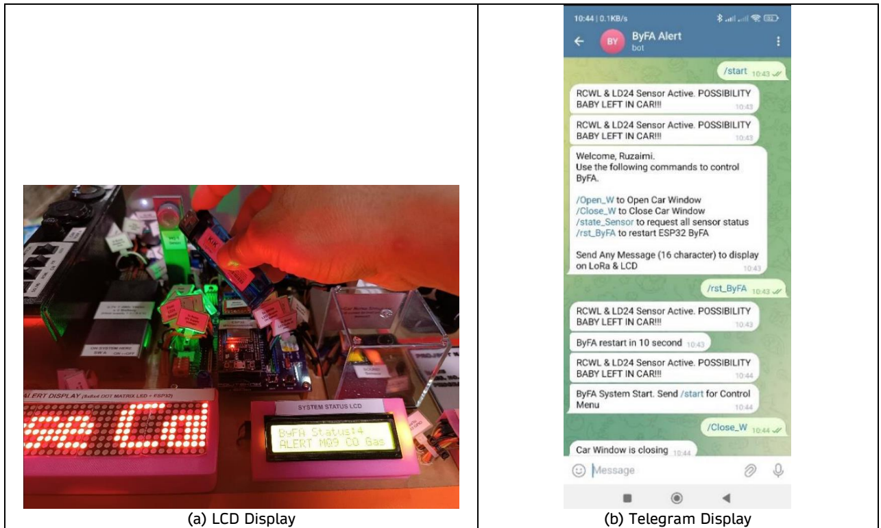
Figure 1.5: Prototype Testing of the ByFAR System using MQ9 Sensor
