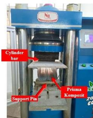
Figure 12 Flexural strength test on composite prisms
