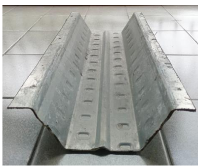
Figure 10 Profile steel sheeting trapezium cross section.
