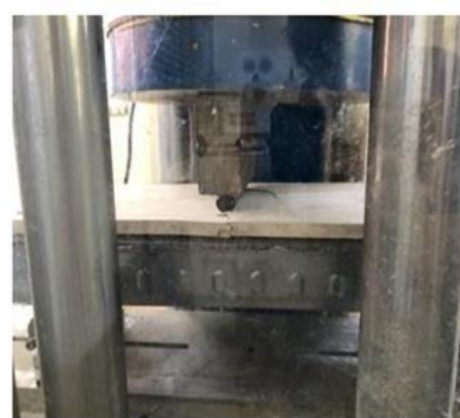
Figure 14 Cylinder bar position for point load
