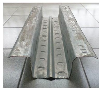
Figure 11 Profile steel sheeting rectangle cross section.
