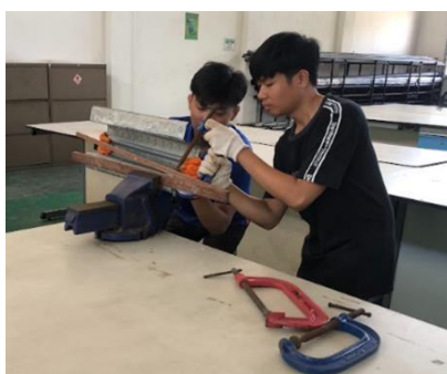
Figure 9 The process of forming a rectangle cross-section.
