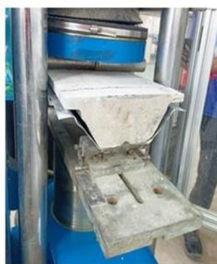
Figure 13 Failure one of the composite prism samples.
