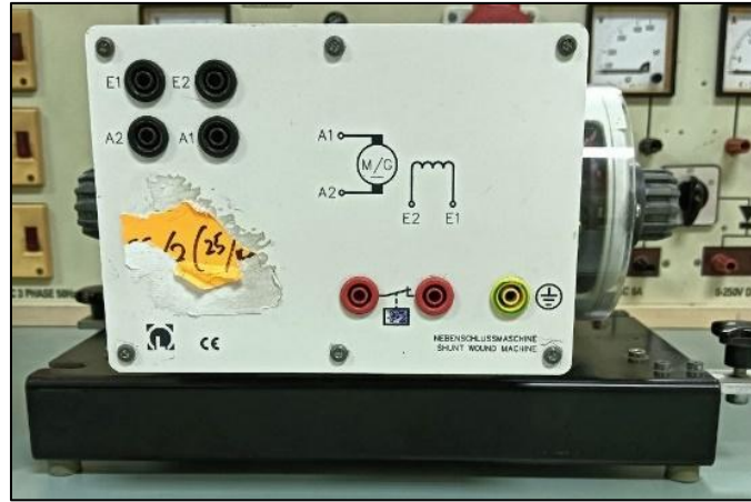
Figure 3.1 0.3kW, 220V DC Shunt Wound Motor Used in Experiment
