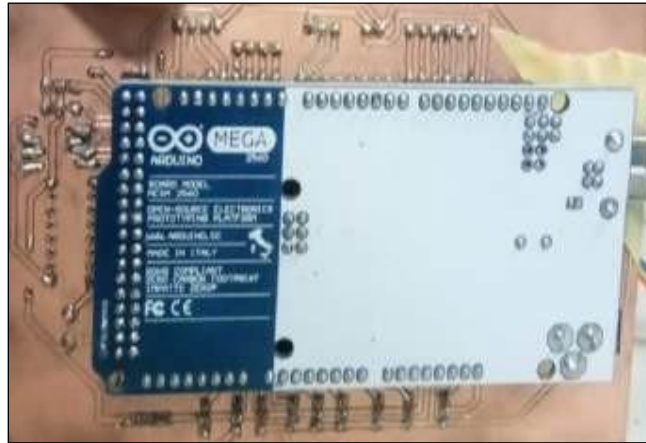
Figure 3: Installation of Arduino Mega 2560 on Schematic PCB
