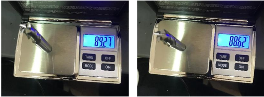
Figure 17: a) Initial Cutter Weight before 1st Cutting Process, b) Cutter Weight after Cutting Process (100th)
