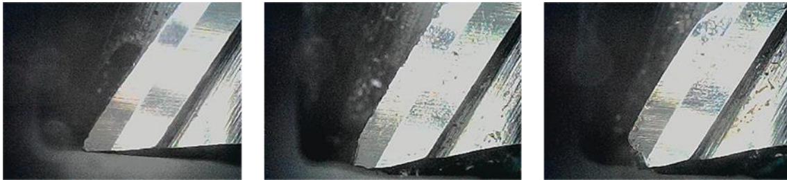
Figure 11: a) Initial condition of sharp cutter (left), b) Cutter condition starting to wear (normal), c) Cutter condition - worn heavily (damaged)
