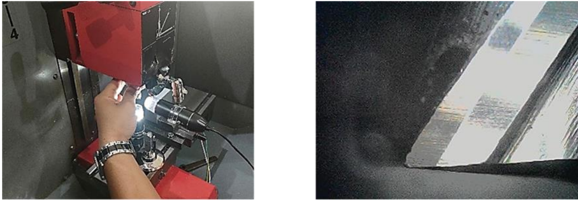
Figure 10: a) The position of the digital microscope during the capture of the tool (left), b) Result of capture
