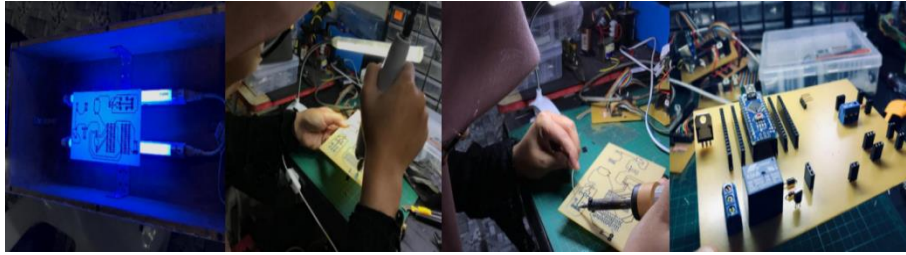
Figure 3 Process to Produce PCB Board
