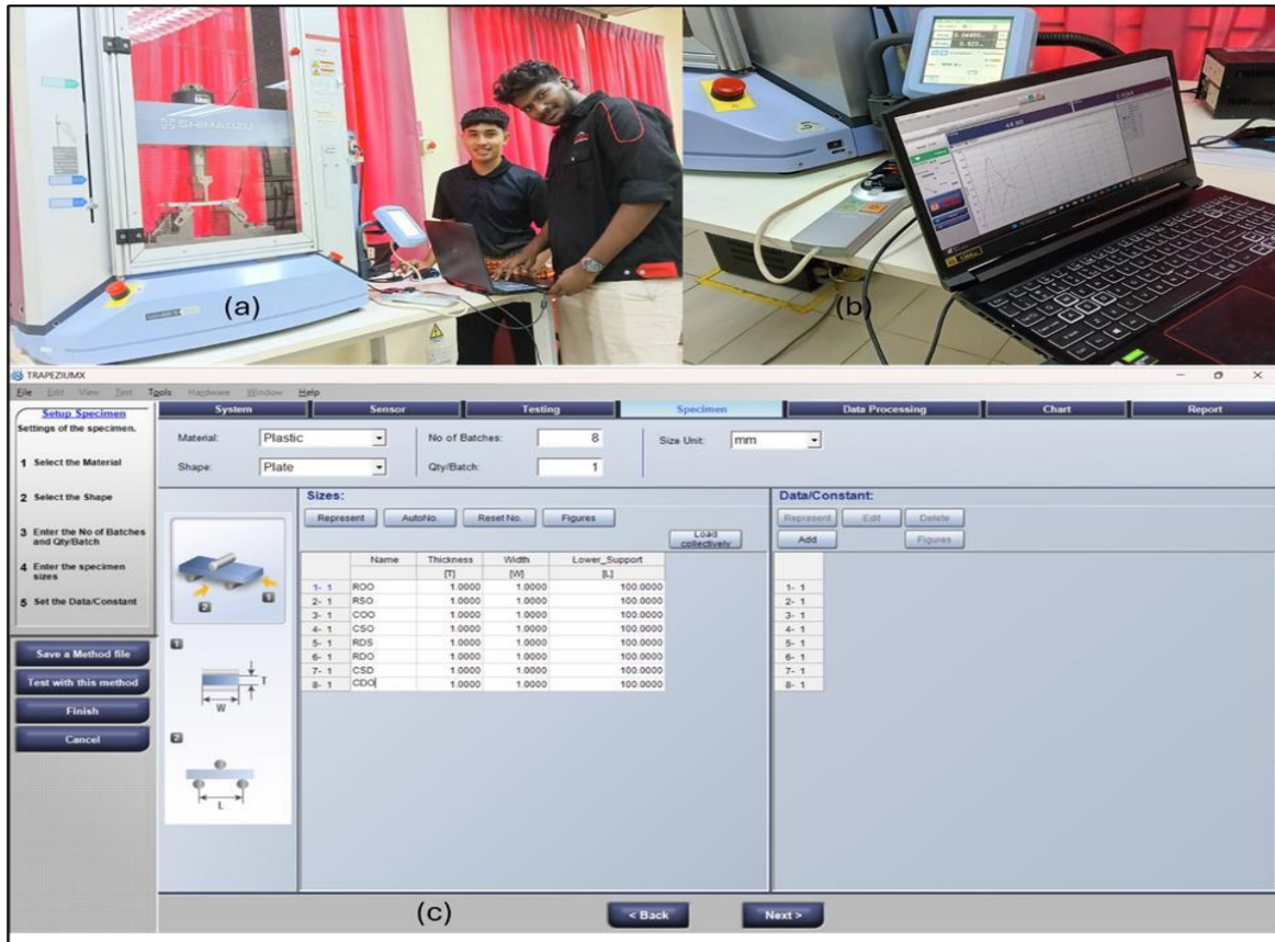
Figure 2. Mechanical test setup. (a) Shimadzu 50 kN universal testing machine, (b) linking Trapezium software to the testing machine, and (c) test specimens' specification setting.
