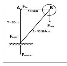
Based on Newton's first law, this situation implies that the net force and net torque (also known as moment of force) on every part of the system are zero (Journal et al., 1924). The balance can be maintained by using the static formula. By reducing the distance of X or Y, stability can be added. In this case, the value of Y is retained when the value of X is reduced so that the robot will be more stable and thus can lift more disks.
