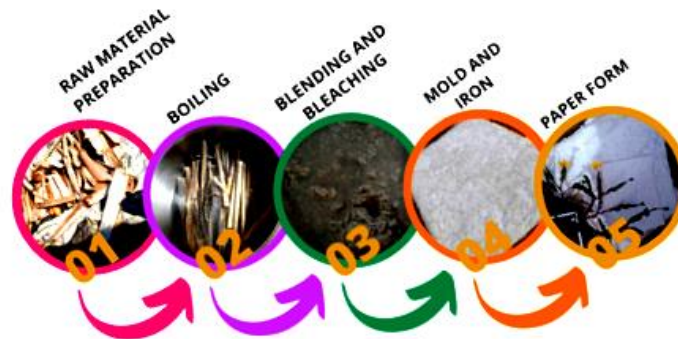
Figure 1.1: The flow process of making drawing paper
